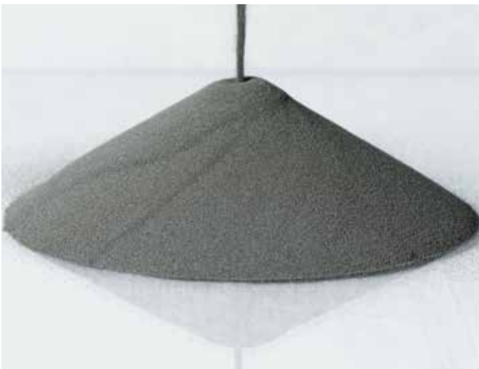
Metal powder for use in additive manufacturing
