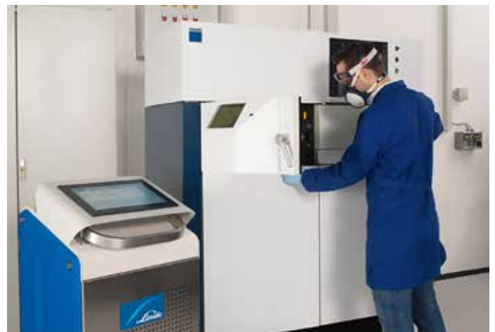
ADDvance® O 2 precision – ensuring the atmosphere of the printing chamber is correct
